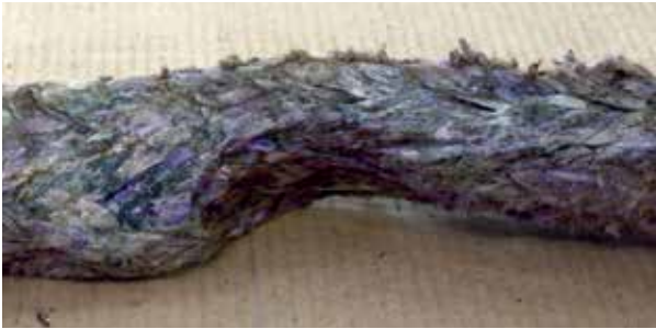
Example of burned and partially melted fiber
