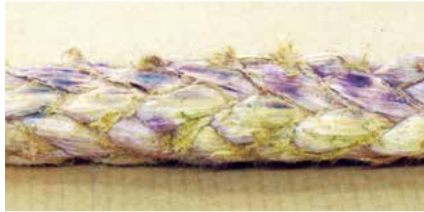
Example of burned and partially melted fiber
