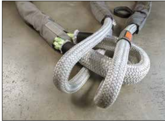
Rigging method of assembly: First slip Component A rope slider sling (lime-green rope) through Component C center link sling 'eyes'
