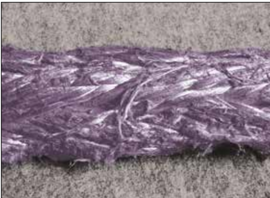
Worn rope surface. Strands appear braided and 'glazed'. Inspection method is visual and compressing (flexing) rope area. If worn rope area cannot "open up" by compression REMOVE FROM SERVICE and replace. If strands area volume is still 75% or more of original and not 'heat-fused' solid, then it is OK to continue to use.
