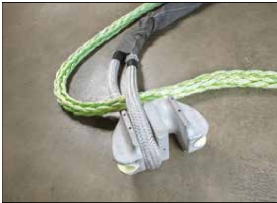
Next, rig one of the eyes of Component C center link into one of the grey channels of Component B load equalizer hardware.
