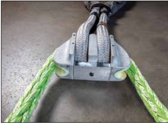
Assemble the 3-part assembly (from bottom up in picture): a. Component A rope slider sling (lime-green rope) b. Component B load equalizer hardware c. Component C center link sling
