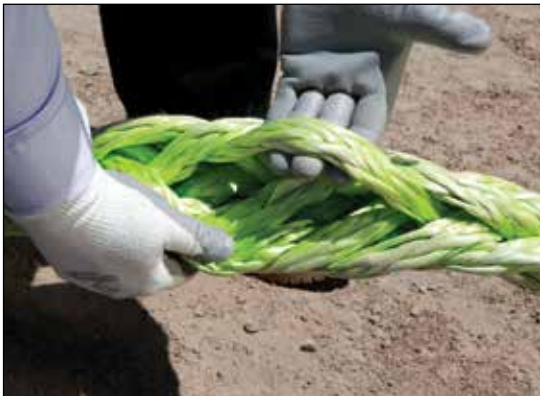
New braided synthetic rope sling. No external rope strand or rope core wear or damage.
