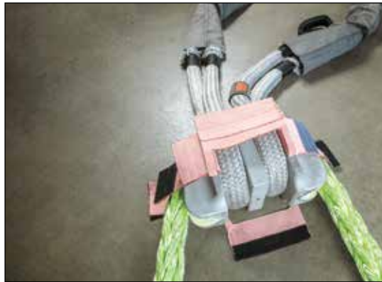
Repeat for the second eye of Component C center link, and position Component A rope slider sling (lime-green rope) in the white channel of Component B load equalizer hardware.
