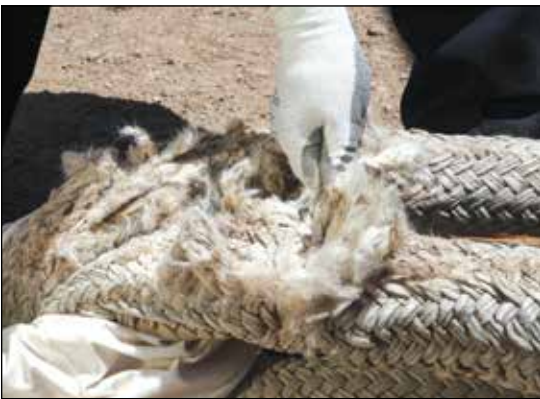
Excessive cutting or wear on braided UHMWPE chafe sleeve. If synthetic rope sling is visible through cut chafe gear, replace sling component.
