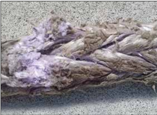
Visual inspection of yarns on rope in this sample shows heavy cutting on two adjacent strands, but only moderate surface abrasion (darker areas on the surface of the strands). This should be removed from service.
