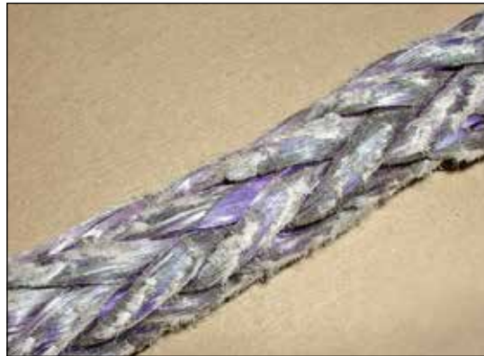
Worn rope surface. Strands appear braided and 'glazed'. Inspection method is visual and compressing (flexing) rope area. If worn rope area cannot "open up" by compression REMOVE FROM SERVICE and replace. If strands area volume is still 75% or more of original and not 'heat-fused' solid, then it is OK to continue to use.
