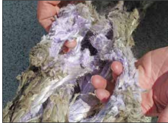
Visual inspection of interior yarns shows wear from abrasion or cutting. This should be removed from service.
