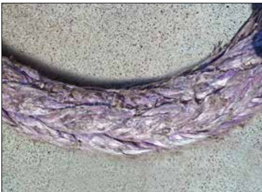
Slight external strand and synthetic fiber yarn abrasion wear and cutting. This rope is good for continued full use.
