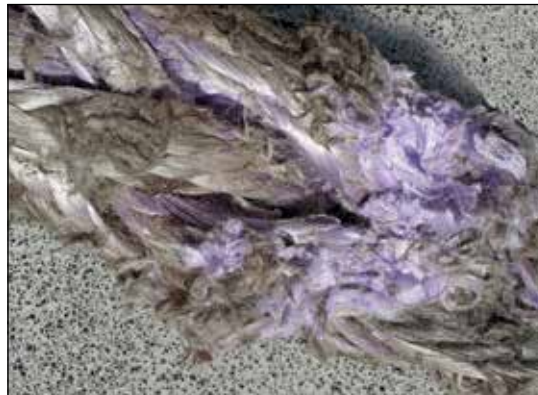
Worn rope surface. Strands appear braided and 'glazed'. Inspection method is visual and compressing (flexing) rope area. If worn rope area cannot "open up" by compression REMOVE FROM SERVICE and replace. If strands area volume is still 75% or more of original and not 'heat-fused' solid, then it is OK to continue to use.
